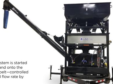
Seed is staged into the holding hopper. When the system is started via the automation, seed flows through the air gate and onto the weigh belt. Using the weight of the seed, the weigh belt—controlled by the automaton—meters to the customer's desired flow rate by changing the speed of the belt.
